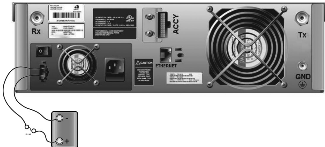
Figure 4-2: Making Connections to a Backup Battery
